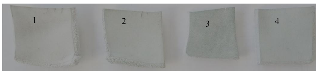
Fig 1. Chromed tanned leather (pickling method: 1 – control; 2 – p TsOH; 3 – p TsOH + EP Oropon DVP 0.05%; 4 – p TsOH + EP Zime SB 0.05%)
