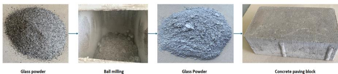
Fig. 1. Preparation scheme for concrete paving block
